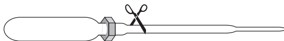
Figure 1: Screw a hex nut onto the pipet and cut off the stem.
