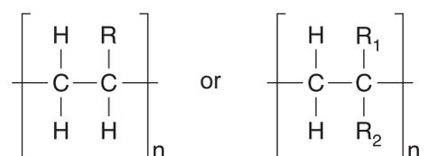
Polyvinyl alcohol (PVAI) has a hydroxyl group as the -R group and polyvinyl acetate (PVAc) has an acetate group. This variation will result in differences in physical properties of the polymers and in cross-linking behavior. Since the cross-linking occurs in part due to hydrogen bonding interactions, the mechanism is similar to water absorption in other non-water soluble polymers.
