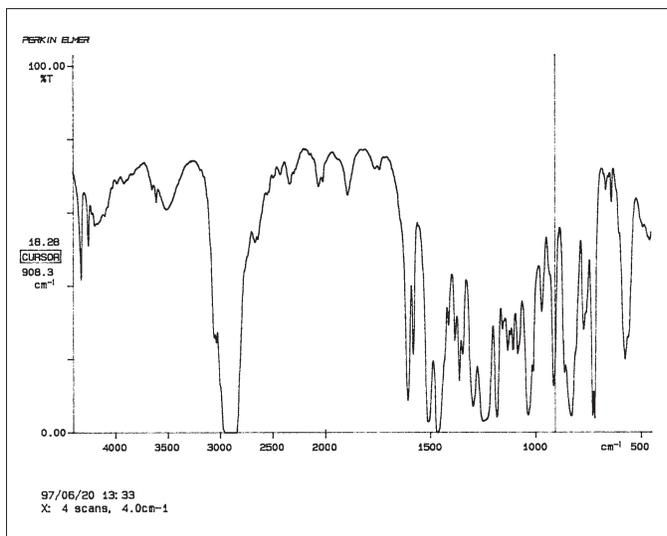
colorless component of two-part epoxy adhesive in polyethylene sandwich
