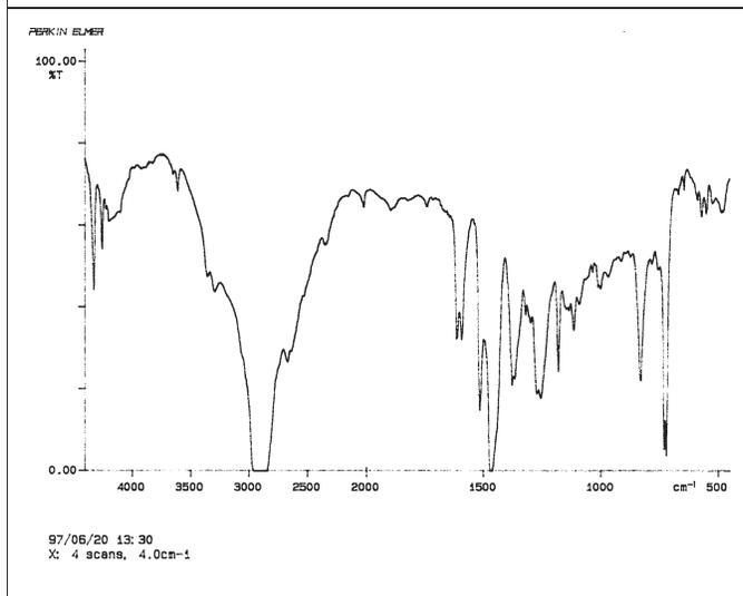
yellow component of two-part epoxy adhesive in polyethylene sandwich
