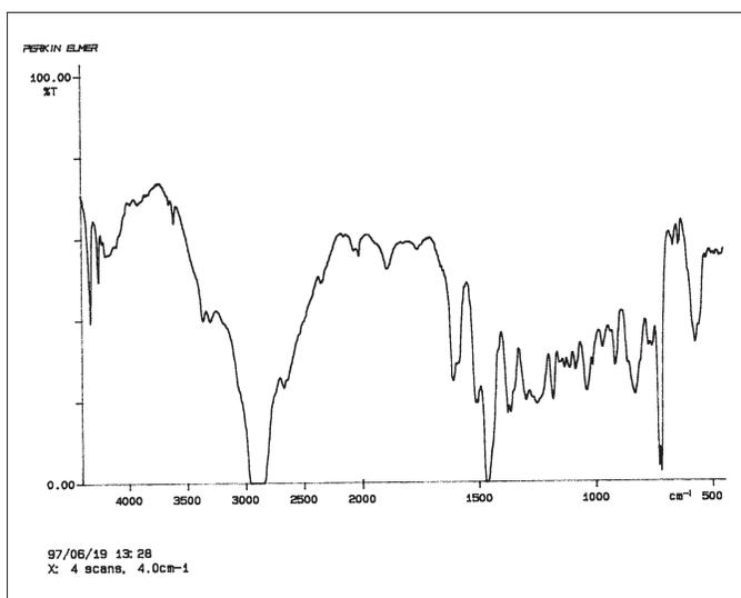
epoxy glue after 4 minutes drying time in polyethylene sandwich
